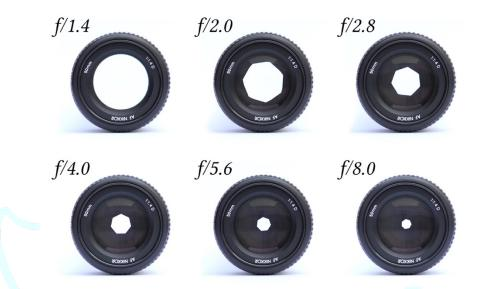
Top: a visual representation of aperture opening sizes and f/stops Photo created by Koeppik, <u>https://en.wikipedia.org/wiki/Aperture#/media/File:Lenses with different apertures.jpg</u> Bottom: Left image uses a shallow depth of field from a small f/stop. Right shows a greater depth of field with a larger f/stop. Note the backgrounds.
